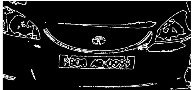
Fig. 11 Morphological Dilation Operation
